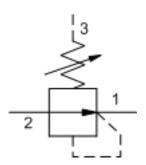
Direct-acting pressure reducing valves reduce a high primary pressure at the inlet (port 2) to a constant reduced pressure at port 1. These valves incorporate a damped construction for stable operation. Note that they should not be used in dead-headed applications since they have no relieving capability.
