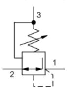
Similar to the PRBB, the PRBC is a direct-acting pressure reducing/relieving valve, but because the valve is open in the transition from reducing to relieving, it provides excellent pressure control and dynamic response for demanding applications. And because they are direct acting with open transition, they offer greater protection in contaminated environments, especially at dead-headed conditions.
