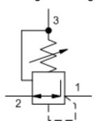
Direct-acting pressure reducing/relieving valves reduce a high primary pressure at the inlet (port 2) to a constant reduced pressure at port 1, with a full-flow relief function from port 1 to tank (port 3). These valves incorporate a damped construction for stable operation in dead headed applications. They're suitable for accumulator circuits since the absence of pilot-control flow results in reduced secondary circuit leakage.
